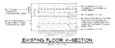
In 2012 the City began to notice that the floor showed significant signs of wear after just four (4) years of use. Large areas of the top slab had eroded 3" in depth, so that that reinforcing steel was exposed and in some places protruding dangerously. Almost 25% of the floor became severely eroded so the City installed an asphalt patch for temporary repair. The push wall also needed repairs, as the structural attachments had pushed through the wall leaving holes.
